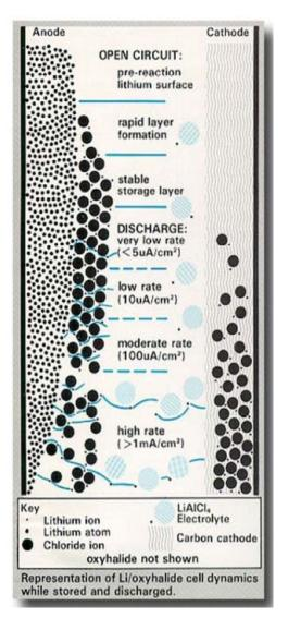
Both of these methods will have an impact on the capacity of the cell. In particular, a low rate discharge tends to increase the normal self-discharge reaction of the cell and reduce the available capacity.
